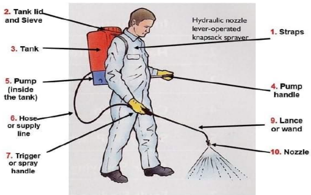
Figure 1.1. Part of knapsack sprayer
