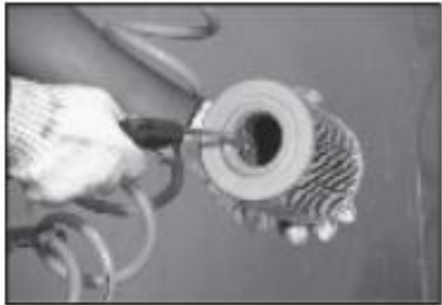
Figure 2.1 air filter cleaning
