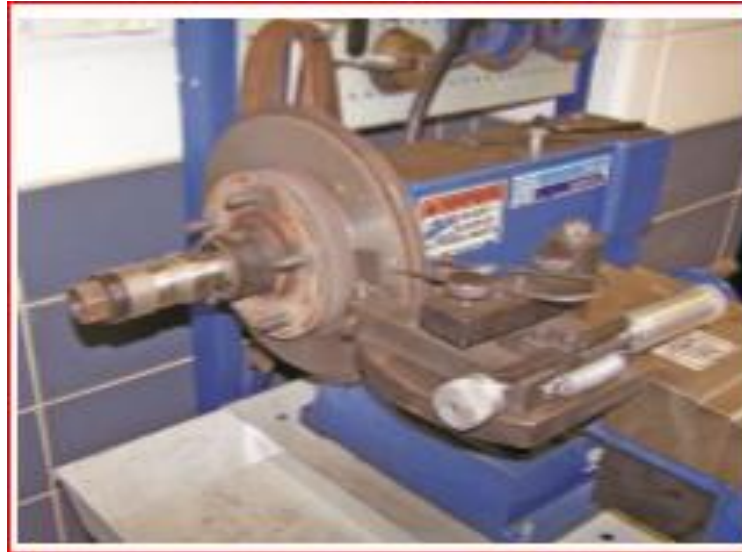
Figure 3:24 A typical bench lathe for resurfacing brake rotor
