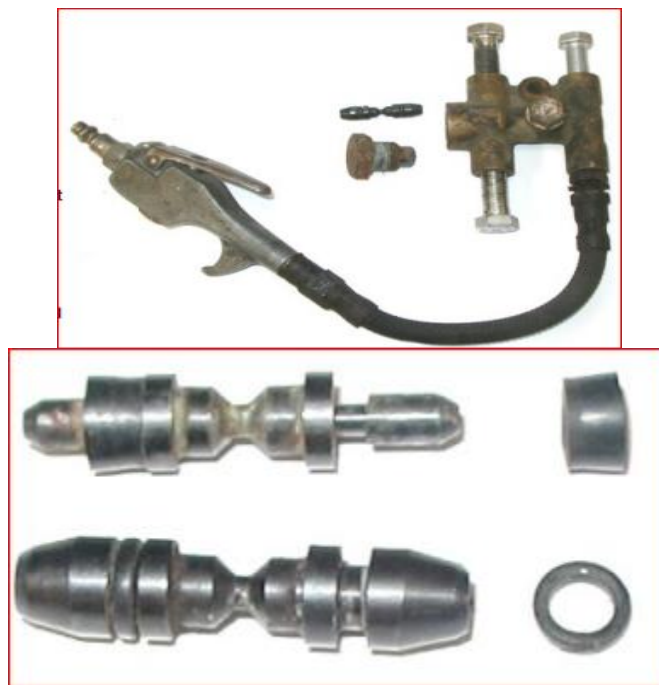
Figure 3:10 coated the piston with rubber grease
