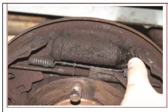
Figure 3:19 check for internal wheel cylinder leaks of drum brake
