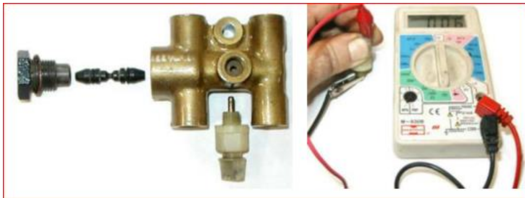
Figure 3:11 tested it by pressing the switch plunger
