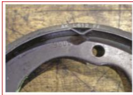
Figure 3:17 Potential brake shoe problems
