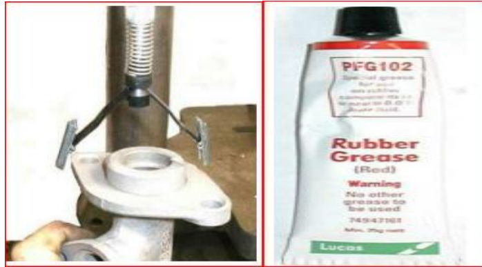
Figure 3:6 Cleaning up the master cylinder casting
