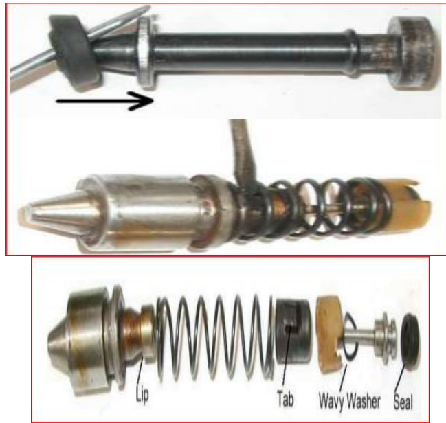
Figure 3:8 Disassembled the master cylinder piston
