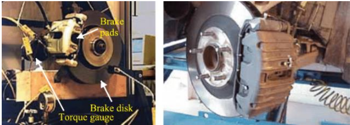
Figure 2:14 Laboratory test stand for testing of disc brake friction characteristics
