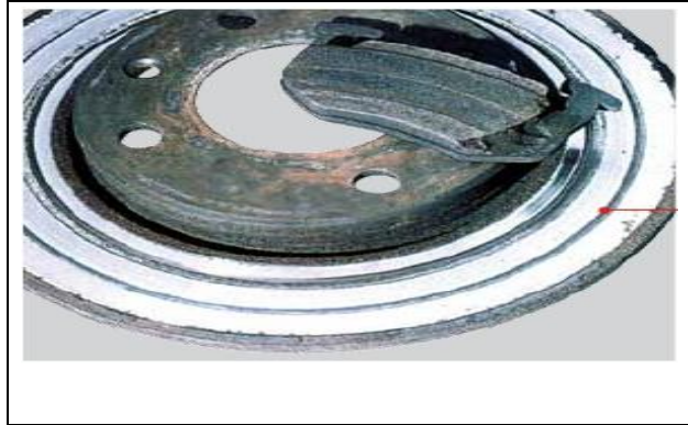
Figure 2:4 Traces of Corrosion Rotor
