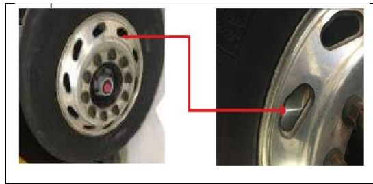
Figure 2:12 Rotor Condition Inspection
