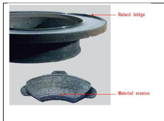
Figure 2:5 A raised bridge at the edge of the friction ring surface
