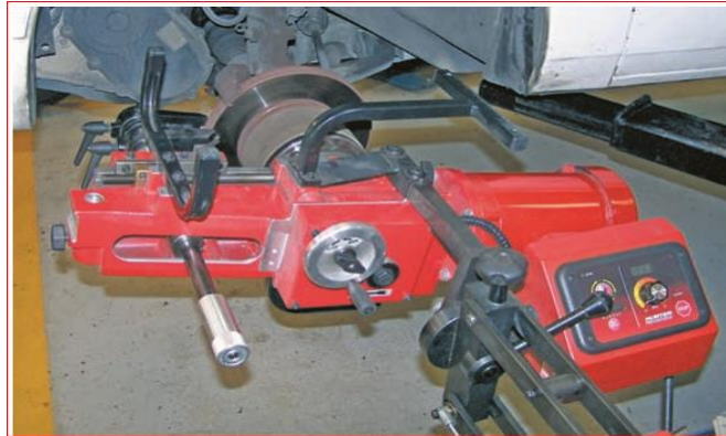
Figure 3:25 An on-the-vehicle brake lathe
