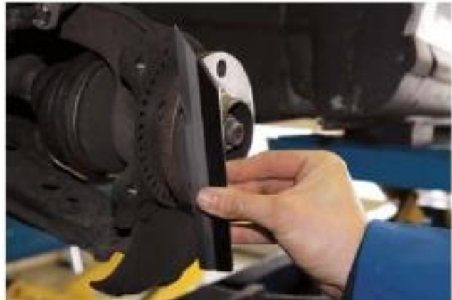
Figure 1:41 Straight edge checking for brake disk flatness
