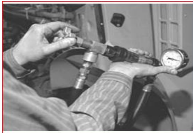
Figure 2:35 close down the flow valve
