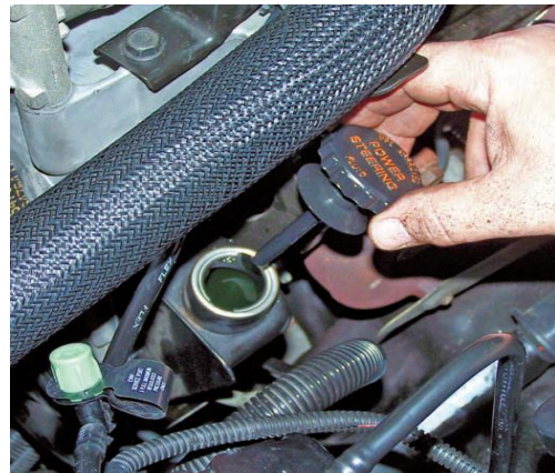
Figure 2:26 Check the fluid level with the dipstick attached to the cap.
