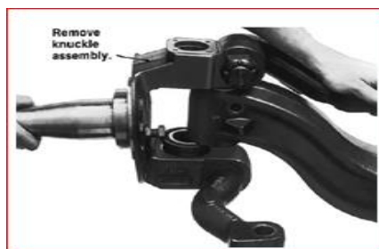
Figure 2:8 with the knuckle pin partially removed
