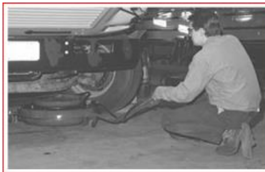
Figure 2:30 Place a drain pan under the steering gear
