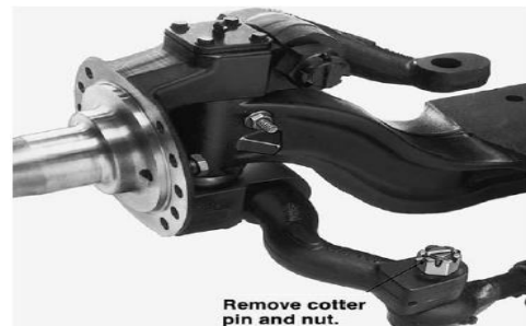
Figure 2: 6 To Remove A Tie-Rod, First Remove The Cotter Pin And Nut.
