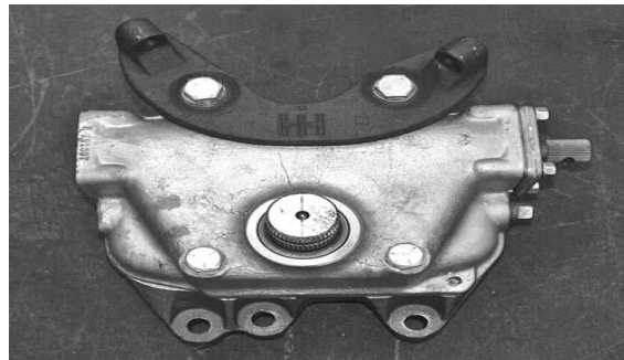
Figure 2:15 When the gear is centered, the sector shaft alignment mark is at a right angle to the input
