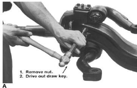
Figure 2:7 To remove the kingpin drive out the draw key
