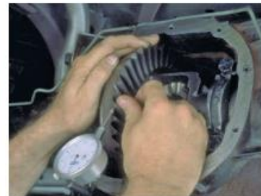
P35-9 Check the backlash and preload of the gearset. Check the backlash by holding the input pinion, rocking the ring gear, and noting the movement on the dial indicator. Adjust the shim pack to allow for the specified backlash. Recheck the backlash at four points equally spaced around the ring gear.
