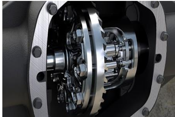
Figure 0.29 Internal parts of limited-slip differential
