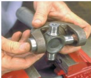
P34-4 Start one cup into the yoke's ear and over the cross's trunnion.
