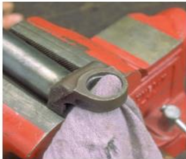
P34-1 Clean any dirt from the yoke and the retaining ring grooves.
