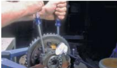
P36-7 Install a dial indicator and position the plunger against the drive side of the ring gear. Set the dial to zero. Using two screwdrivers, pry between the differential case and the housing. Observe the reading.
