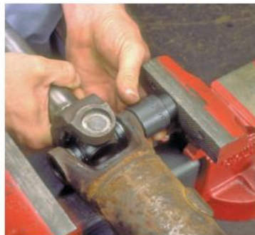
P33-5 Place the large socket against one vise jaw. Position the drive shaft yoke so that the socket is around a bearing cup.
