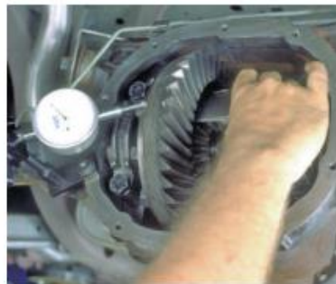
P35-5 Mount a dial indicator to the housing so that the button of the indicator touches the face of the ring gear. Using two screwdrivers, pry between the shims and the housing. Pry to one side and set the dial indicator to zero, then pry to the opposite side and record the reading.
