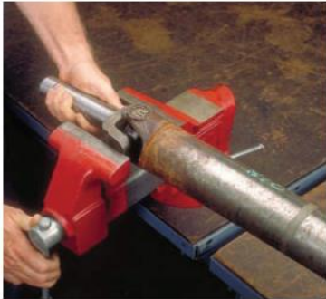
P33-1 Clamp the slip yoke in a vise and support the outer end of the drive shaft.
