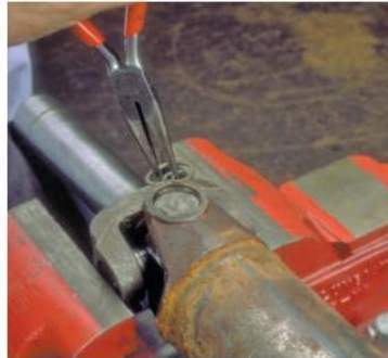
P33-2 Remove the lock rings on the tops of the bearing cups. Make index marks in the yoke so that the joint can be assembled with the correct phasing.
