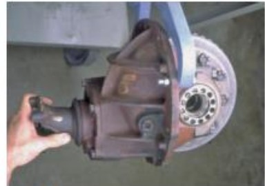
P36-6 Seat the bearings by rotating the pinion several times each time the adjusters are moved.
