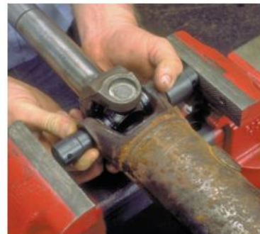
P33-6 Position the other socket to the center of the bearing cup opposite to the one in line with the large socket.
