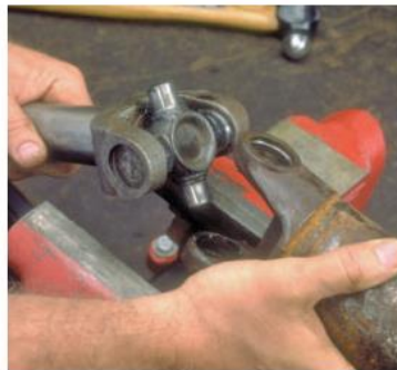
P33-8 Separate the joint by turning the shaft over in the vise and driving the cross and remaining bearing cup down through the yoke with a brass drift and hammer.
