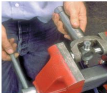
P34-5 Carefully place the assembly in a vise or U-joint bearing press and press the cup partially through the ear.
