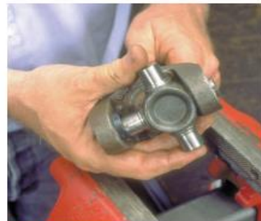
P34-6 Remove the shaft from the vise and push the cross toward the other side of the yoke.
