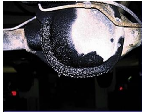
Figure 0.1 Differential ready for removal and overhauling
