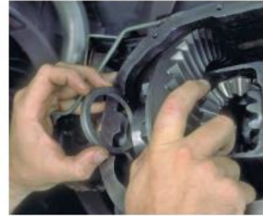
P35-3 Install service spacers that are the same thickness as the original preload shims between each bearing cup and the housing.
