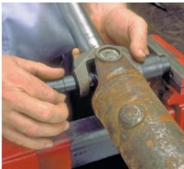
P33-4 Select a second socket that can slide into the shaft's bearing cup bore—usually a 9/16-inch socket.
