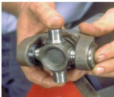
P34-7 Start a cup into the yoke's ear and over the trunnion.
