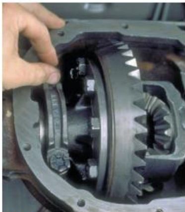
P35-4 Install the bearing caps and finger tighten the bolts.
