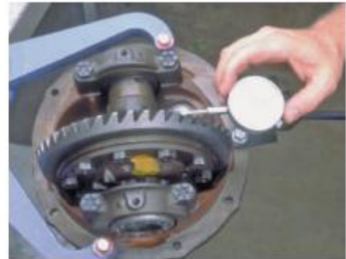
P36-9 Check the backlash by rocking the ring gear and noting the movement on the dial indicator.
