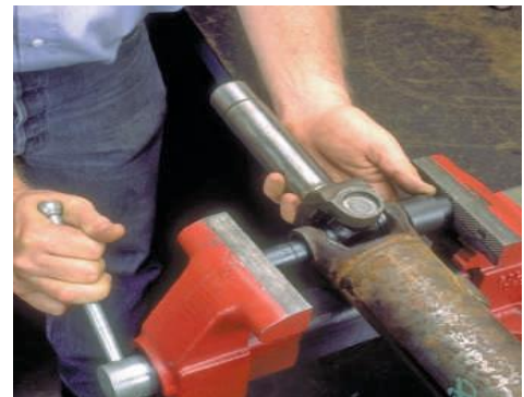
Figure 0.7 Removing U-joint by using vise
