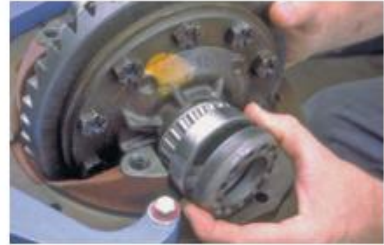
P36-3 Install the bearing cups and adjusting nuts onto the differential case.
