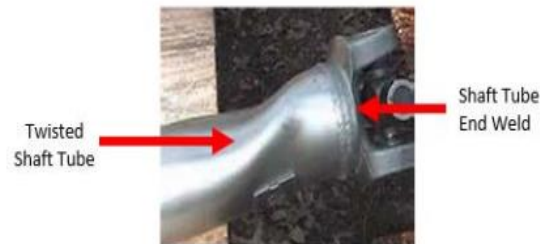
Figure 0.17 Inspection of Driveshaft Tube
