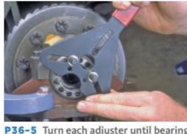
P36-5 Turn each adjuster until bearing free play is eliminated with little or no backlash present between the ring and pinion gears.
