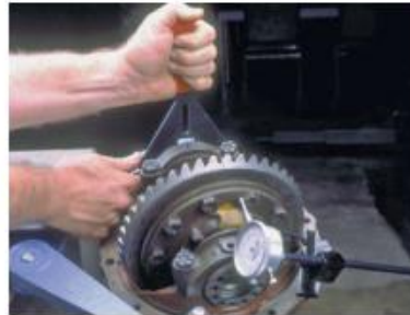
P36-8 Determine how much the preload needs to be adjusted and set the preload by turning the right adjusting nut.
