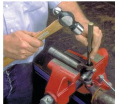
P33-9 Use a drift and hammer to drive the joint out of the other yokes.
