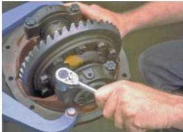
P36-4 Snugly tighten the top bearing cup bolts and finger tighten the lower bolts.
