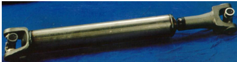
Figure 0.10 Propeller shaft U-joint and slip joint
