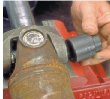
P33-3 Select a socket that has an inside diameter large enough for the bearing cup to fit into; usually a 1/4-inch socket works.
