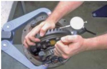
P36-10 Adjust the backlash by turning both adjusting nuts in equal amounts so that the preload adjustment remains unchanged.
