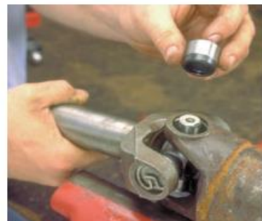
P34-9 Position the joint's cross in the drive shaft yoke and install the two remaining bearing cups.
