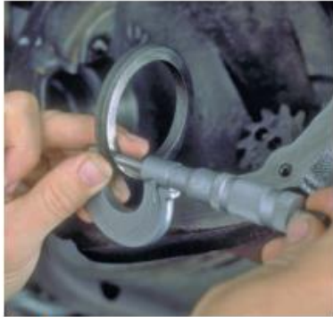
P35-1 Measure the thickness of the original side bearing preload shims.
