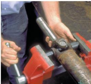
P33-7 Carefully tighten the vise to press the bearing cup out of the yoke and into the large socket.
