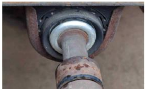
Figure 0.15 Inspection of Yoke End Fittings
