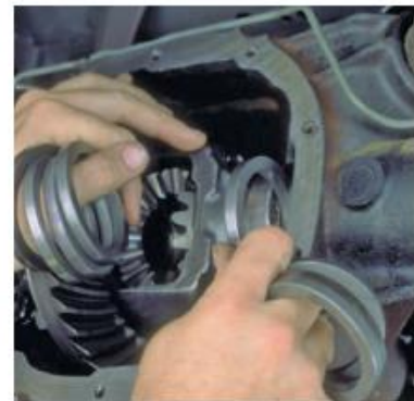
P35-6 Select two shims with a combined thickness to that of the original shims plus the indicator reading, then install them.
