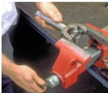
P34-8 Place the shaft in the vise and tighten the jaws to press the bearing cup into the ear and over the trunnion. Then install the snaprings. Make sure they are seated in their grooves.
