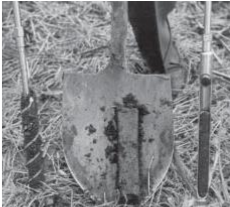
Figure 1.3 A soil probe, auger, spade and knife should be used in sampling soils
