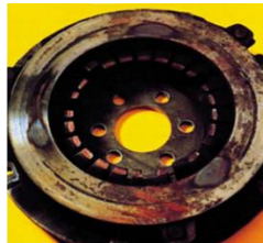
Hot spots of clutch slip or oil onto the clutch facing.
