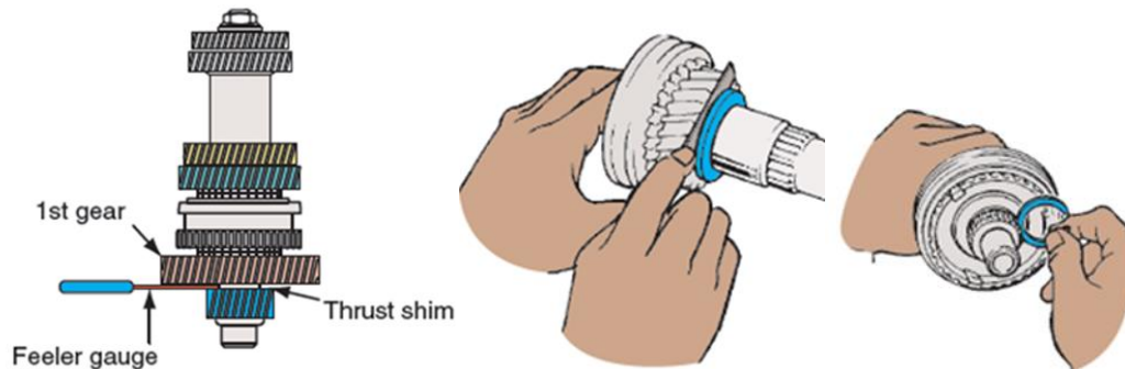
Figure 0.13: Check thrust clearances between gears and synchronizer assembly
