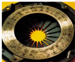
Heavy chatter marks oil or grease onto the clutch facing.
