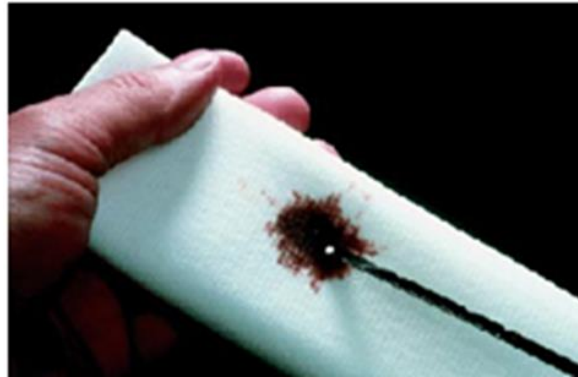
Figure 0.3: Condition of automatic transmission fluid
