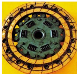
Deep scoring in the friction material on the flywheel side flywheel was not resurfaced or replaced during a previous repair
