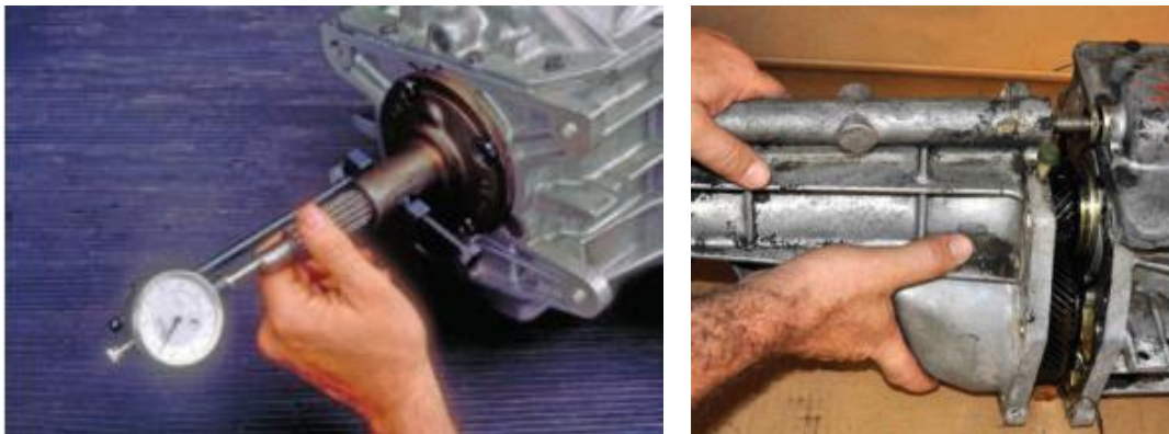
Figure 0.8: Use of a dial indicator to measure the endplay of the shafts before disassembling the unit (left) and sliding the extension housing off the output shaft (right)
