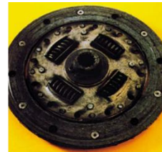
Friction material worn down to the rivets.
