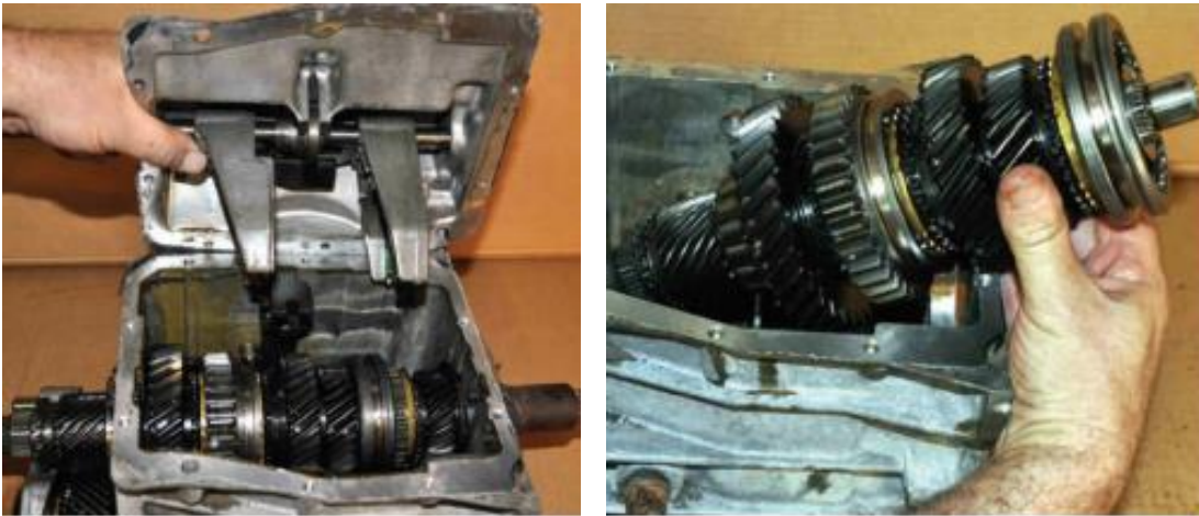
Figure 0.9 Remove the top cover and the shift linkage and Lift the output shaft from the case and then
