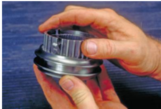
Figure 0.11: Synchronizer mechanism and shift hub check
