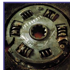
A destroyed torsional damper by driving at too low an engine speed
