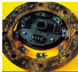
A broken cushion segment caused by a missing or defective pilot bearing.
