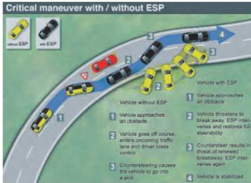
Figure 1.11 effects of a stability control EPS
