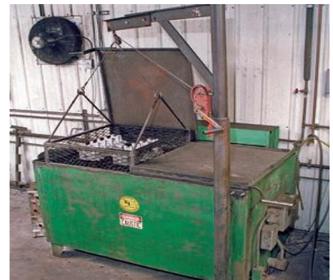
Figure 1.2-14 cold soak tank
