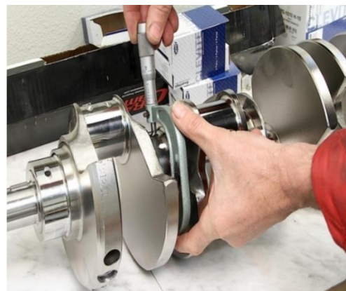
Figure 3.21 Connecting Rod journal Diameter
