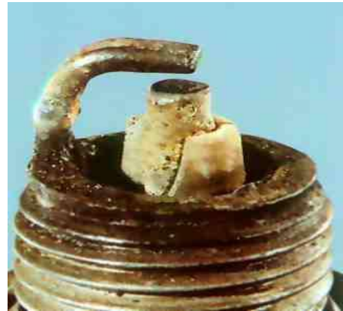
Figure 3: 21 Severe Detonation of Sparkplug
