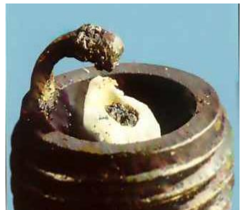
Figure 3: 26 Sustained Pre-ignition in sparkplug
