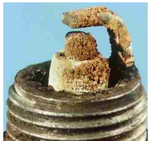
Figure 3: 23 Ash Deposits in the Spark Plug
