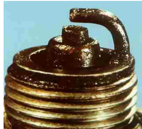
Figure 3: 24 Oil Fouled Sparkplug
