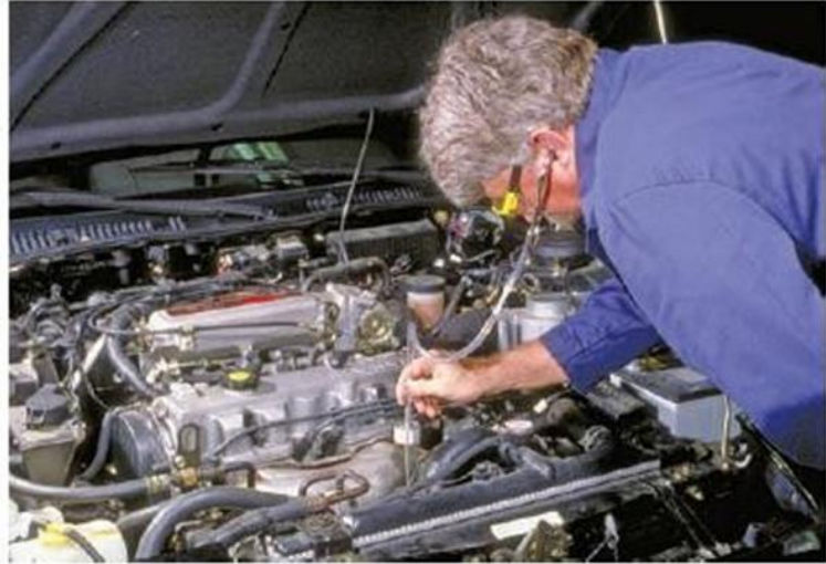
Figure2:3 Technician Uses Mechanical Stetoscope
