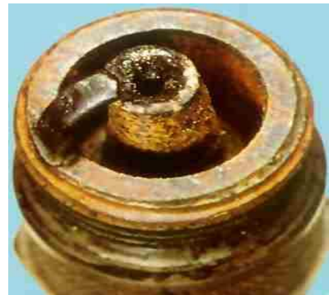
Figure 3: 25 Initial Pre-ignition in Sparkplug
