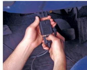
P24-6 Connect the scan tool to the DLC.
