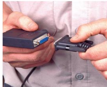
P24-5 Select the proper scan tool adapter for the vehicle's DLC.
