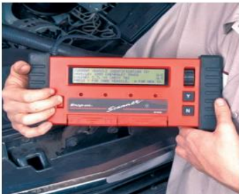
P24-4 Enter the vehicle's model year and VIN code into the scan tool.
