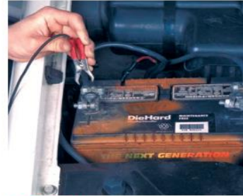
P24-3 Connect the scan tool power leads to the battery or cigar lighter (depending on the design of the scan tool).
