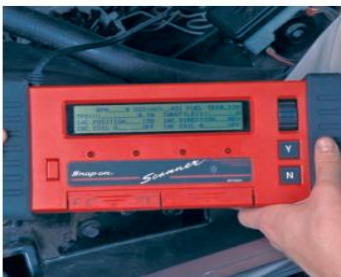
P24-7 Retrieve the DTCs with the scan tool. Interpret the codes by using the service manual.
