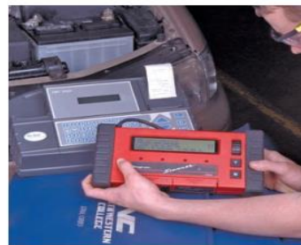
P24-8 Start the engine and obtain the input sensor and output actuator data on the scan tool. If a printer for the tool is available, print out the data report.
