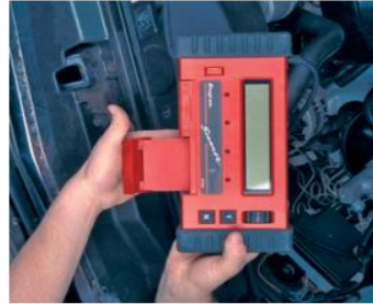
P24-2 Install the proper module for the vehicle and system into the scan tool.
