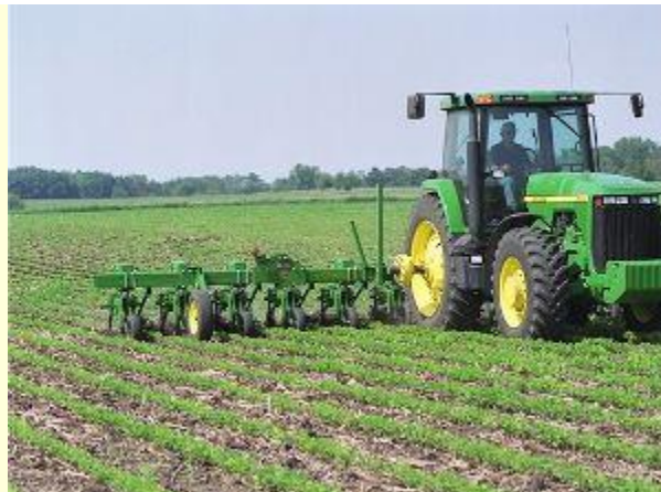
Figure.1.4. a tractor and row crop cultivator working in soybeans planted with a conservation tillage system
