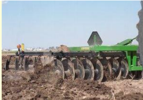
A close-up view of a disk harrow in the field Figure.1.2 Disk harrow
