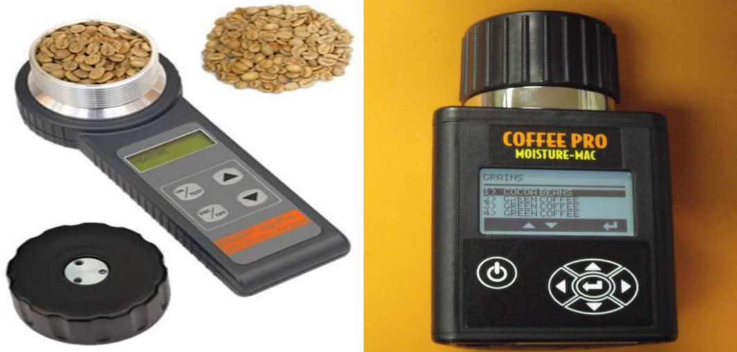
Figure 3.2. Moisture meters used to check coffee moisture
