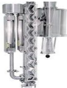
Laboratory zigzag classifier
