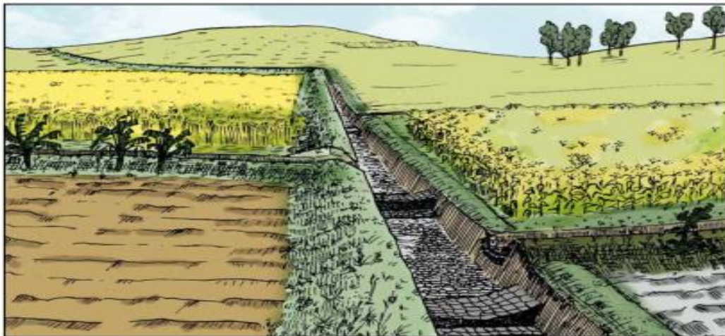
This is a typical artificial waterway in an area with land scarcity. Therefore, it has been dug deep into the soil, with steep borders and a stone pavement with intermittent small checkdams at the bottom. At the top, a cutoff drain leads into the waterway from the left side, while, graded bunds are led into it from the cultivated land, alternating from each side.
